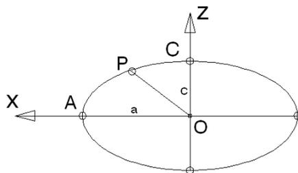
$$\frac{x^2}{a^2} + \frac{z^2}{c^2} = 1 \quad \text{bzw.} \quad z = +\frac{c}{a} \sqrt{a^2 - x^2} \quad \text{und} \quad \overline{OP} = \sqrt{x^2 + z^2}.$$
